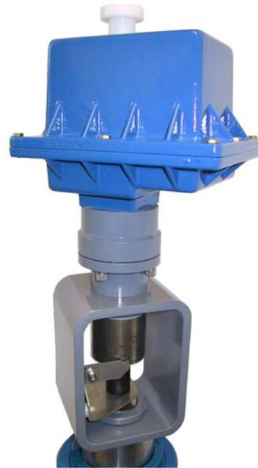
**Simply remove the stainless operating lever and mount our 24 vDC electric actuator when you want to automate. The unit may be powered with a small solar array and will accept 4 different analog command signals. The actuator may be safely installed or removed while the choke is throttling and under pressure.**
