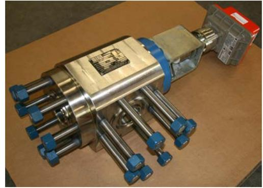
3-1/16"-15M all Nickel Alloys, "HH", PSL 3G (extra long 718 inlet studs for instrument flange)
